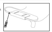
Remove tray and flip upside down on a flat working surface. Position brackets on tray, lining up with marks. Using brackets as a template, mark where slots in brackets make contact with tray.
