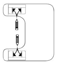
3. Remove brackets from tray, drill one hole through tray in approximate center of each marked slot area. Countersink holes.
