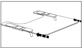
2. The long slots in the brackets allow for considerable adjustment. Center tray on chair, adjust brackets to fit against the edge of armrests. Tighten screws that hold brackets to tray.
