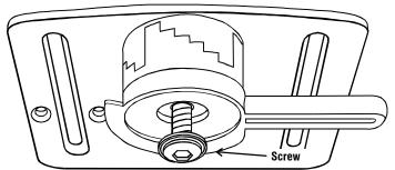
Loosen the screw in each clamp that goes through the Handle, it's on the bottom of each clamp assembly. This allows the clamps to be adjusted to the *HEIGHT* of the armpads.
