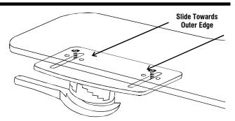
3. The long slots in the clamps allow for considerable adjustment. Slide the clamp assemblies to the widest position on the tray.
