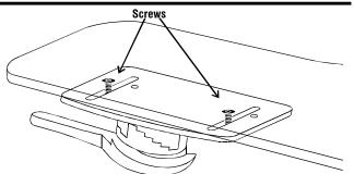
1. Loosen the screws that hold the Top Drop Clamps to the tray. This allows the clamps to be adjusted to the *WIDTH* of the armpads.
