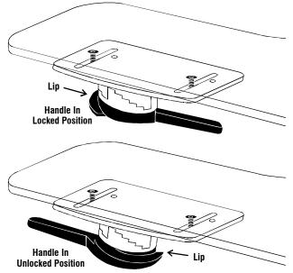
Rotate the clamp Handles to the UNLOCKED position, which puts the little lip on the handle piece towards the OUTSIDE of the tray. (Later, when you rotate the Handles to the locked position, this lip will fit under the armpad to hold the tray in place.)
