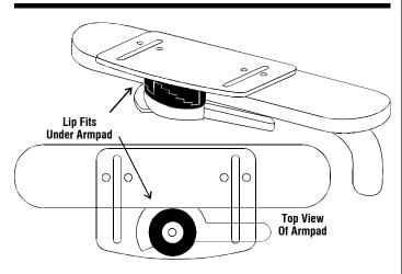
7. Loosen the screw so the Handle and the Step Collar hang down below the bottom edge of the armpad. Rotate the Handle into the *LOCKED* position, which puts the lip on the Handle piece under the armpad. Push up on the Handle from the bottom with one hand, and rotate the Step Collar with your other hand. Rotate the Step Collar into different positions, and find the right "step" that allows the lip on the Handle to fit snug under the edge of the armpad.
