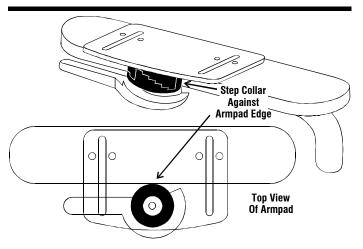
5. Center the tray on the chair, and adjust the clamp assemblies so the Step Collar (the tall round piece with little "steps") fits snug against the side of the armrest. Tighten the screws that hold the clamps to the tray, the screws you loosened in Step 1. The screws should be tightened so the tops are flush with the surface of the tray.
