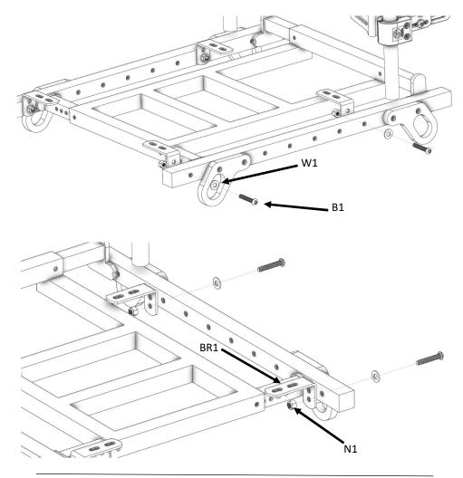
**Step 2**: Attach seat base by passing bolt B2 through the bracket BR and into
