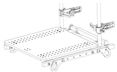
**Step 4**: Attach seat to newly installed seat base.
