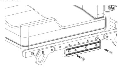
Step 2: Install using bolts B1 and tighten securely with nuts N2.
