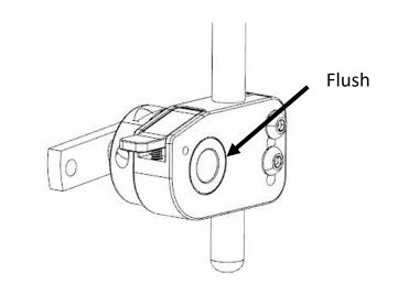
D. Slide Collar snugly against the Washer and Flip Down Clamp and ensure that the Axle does not protrude. Tighten Collar Bolts.
