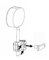
B. Determine a location along the pan located on the wheelchair frame to attach the Mount. And attach with 5/16 bolts and nuts and reinstall clamp.
