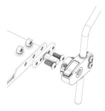
C. Ensure that the Axle is flush with the Flip Down Clamp before tightening collar bolts.
