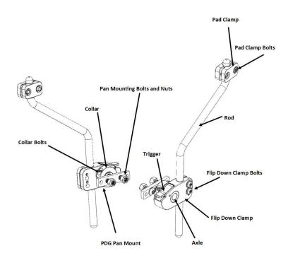
The Adductor is configured as either a *Long Arm* or *Short Arm* model. The illustration below indicates the difference.
