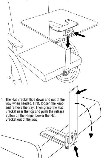
If more room is needed between the tray and the user, the tray may be rotated 180°. Remove the 4 bolts from the top of the tray, rotate the tray, and replace the 4 bolts. The Knob must face away from the user.
