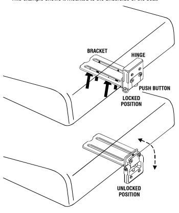
2. Mount the long Flat Bracket to the Hinge. Use 2 bolts and washers supplied.
