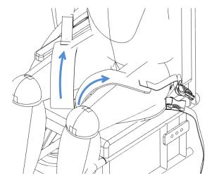
**Step 3**: Fasten buckles around either leg of the user and pull strap to tighten.
