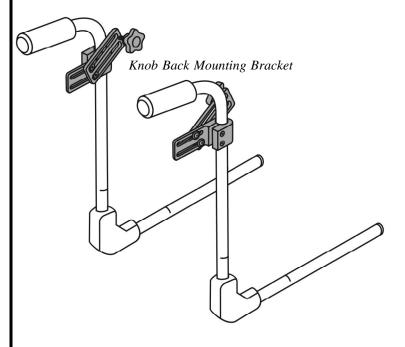
**Step 3**: Install Knob Back Mounting Brackets on the back canes of the chair. Use the spacer for 7/8" tubes.
