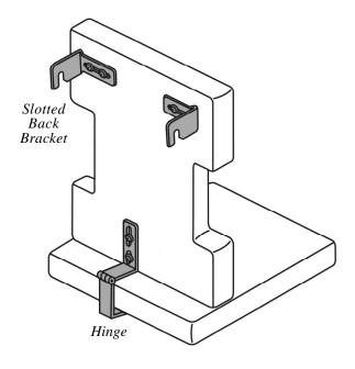
**Step 1**: Install the Hinge.
