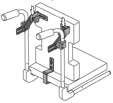
**Step 4**: On the back cushion, adjust the Slotted Back Brackets so they sit on the Knob Back Mounting Brackets. Tighten them onto the back cushion. Tighten the Knob so it holds the Slotted Back Brackets in place, but leave the Back Mounting Brackets loose enough to be adjusted later.
