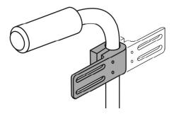
To achieve maximum growth adjustment, the Back Mounting Bracket can be installed on the cane in either direction.
