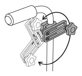
To achieve maximum angle and growth adjustment, the Knob Bracket can be rotated around, and slid back and forth in the slots.
