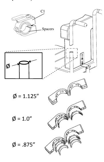
**Step 4**: Attach C1 to wheelchair. Place as shown below. Tighten fasteners.
