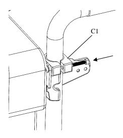
**Step 5**: Rotate latch on C1 to remove back from wheelchair.
