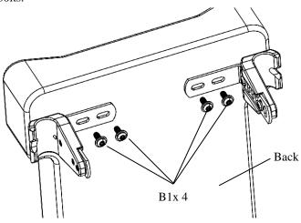
Step 2: Adjust H1 to fit wheelchair. Tighten bolts.
