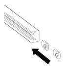
**Step 2**: Attach Adapter using M8 Flat Head Bolts. Position along track and tighten bolts.
