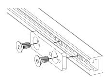
Step 3: Attach Swing away hinge using Socket Head Bolts
