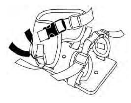
**Step 2**: Adjust the 2 straps with the cam lock buckles on the side of the heel.
