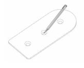
Step 3: Place Mounting Plate back in Body and secure with included bolts and nuts.
