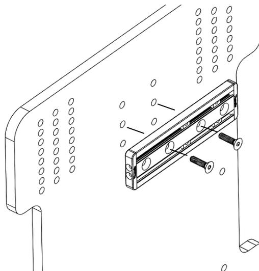
**Step 2:** Attach Headrest Clamp (not included) using bolts B2 threaded into nuts N1.
