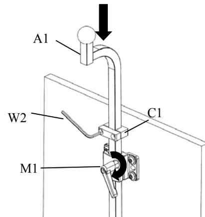
3. Place C1 in desired position and tighten bolts with wrench W2.
