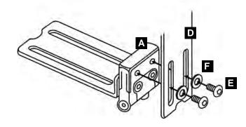
Use Extender Bracket for extra adjustment in any direction.
